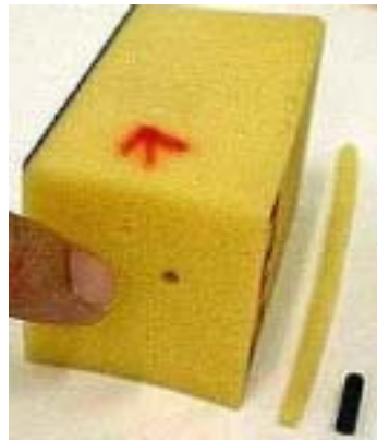
Impact perforation of urethane foam (left), removed plug (middle), \phi 4 mm projectile (right)
